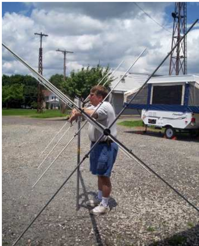
Assembly of the 6 Meter Quad can be tricky since it is a 3 dimensional antenna, Lou WX3I (standing) kept things together as Susan K3SUE and Dan KA3KHR untangled the wire-loop elements. Photo by KA3QOT
