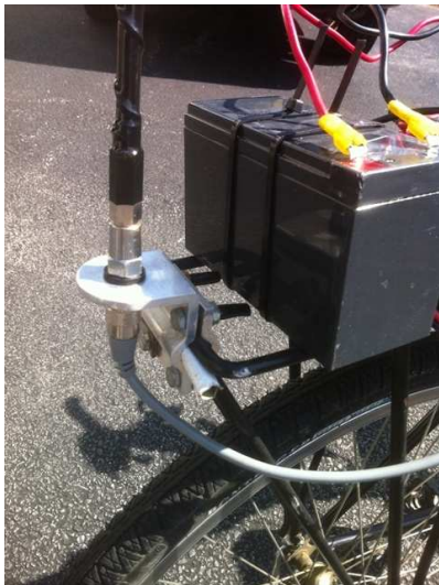
Figure 24 - Antenna mount and battery. The transceiver body is between the battery and the back of the seat.
